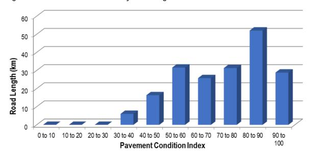
Figure 3: Pavement Condition Index by Road Surface
