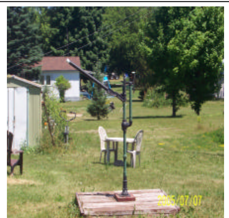
Fig 3: Original pump well
