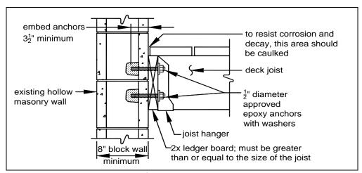
Note: Ensure anchors into solid masonry of block or through bolt with a carriage bolt
