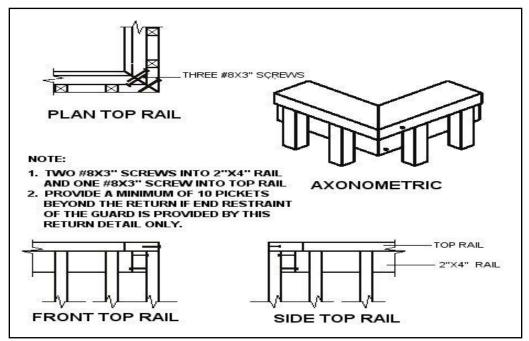
Note: Posts required at opening and change of direction if less than 10 pickets
