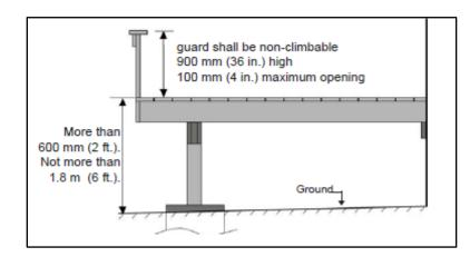
The OBC requires that a guards be installed on walking surfaces on each side that is not protected by a wall where [OBC Division B 9.8.8.1(1)]:
