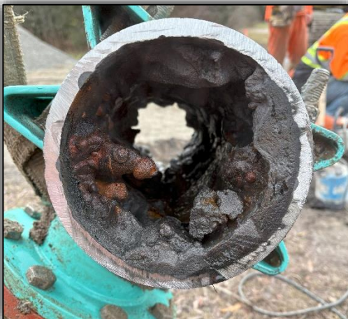
Buildup of corrosion in the existing cast iron pipe – this pipe is abandoned and no longer in use.
